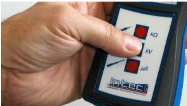
5.) Press and release the kV test button (14).
