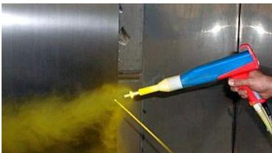
4.) Hold the antenna (8) directly in the powder cloud exiting the jet nozzle of the spray gun.
