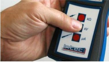
3.) Press the kV (14) **or**  $\mu$ A button (15) on the device.
