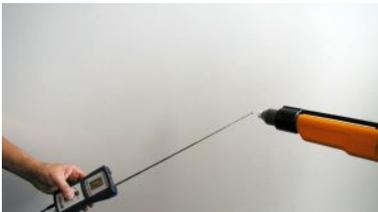
4.) Slowly approach the high-voltage source (spray jet electrode) with the antenna from a distance of around 30 cm.
