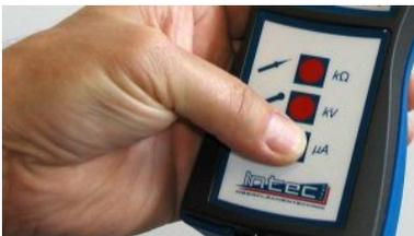
3.) Press and release the  $\mu\text{A}$  test button (15).
