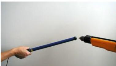
6.) During this time, hold the kV probe (2) with the spherical measuring head directly against the high-voltage source (spray jet electrode).
